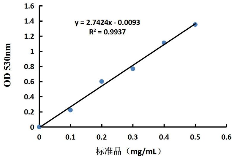
2、可溶性果胶含量(mg/g 重量)=[( $\Delta A + 0.0093$ ) $\div 2.7424 \times V_1$ ] $\div (W \times V_1 \div V) \times D$
